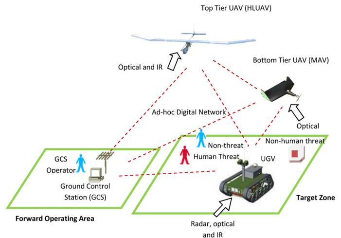
**Figure 1.** SATURN's high-level architecture. UAV, UGV: Unmanned aerial and ground vehicle, respectively. HLUAV: High-level UAV. MAV: Micro air vehicle.
